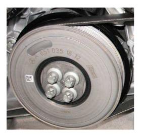
For those vehicles on which an Oliva Torras mount and Drive kit has been installed, it is necessary to mount a new added pulley to drive the compressor.
